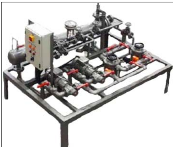
Picture 20 – Oil pump units: with self cleaning filter and oil heaters (electrical and/or steam)
