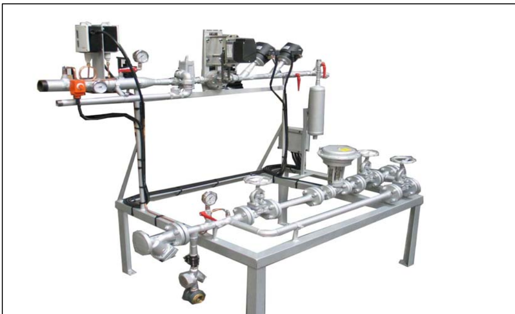
Picture 26 – Oil Handling Unit preassembled on a self standing frame
