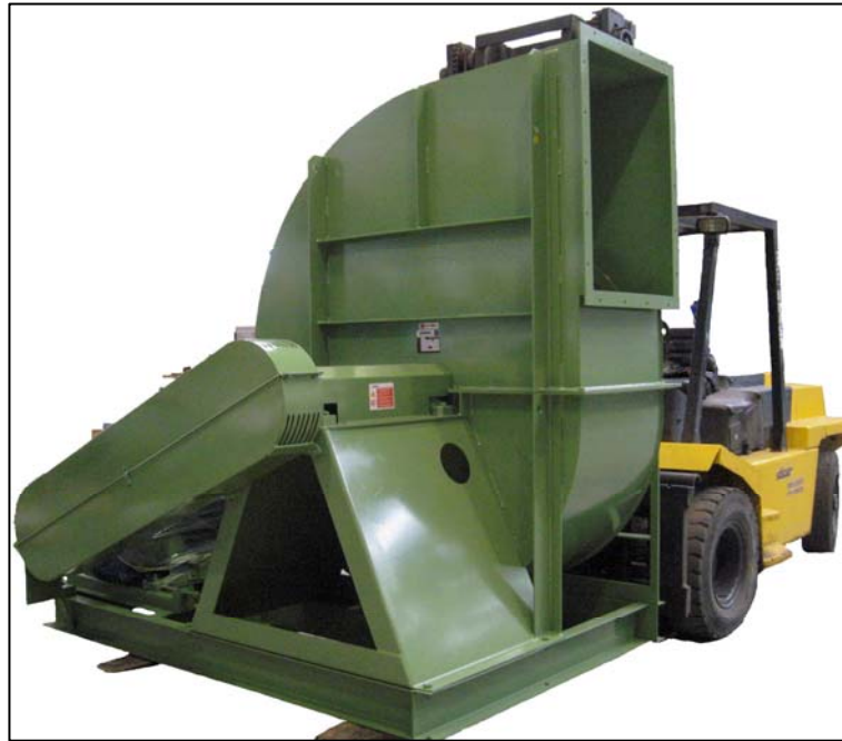
Picture 10 – Draught fan with indirect motor coupling
